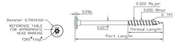
Figure 1. FastenMaster FlatLOK Fasteners
