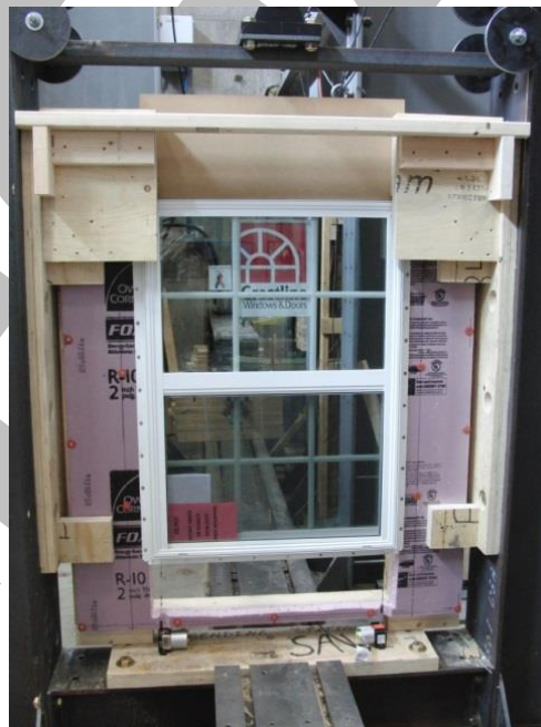
FIGURE 3. STRUCTURAL LOADING – FASTENER/FLANGE CAPACITY
