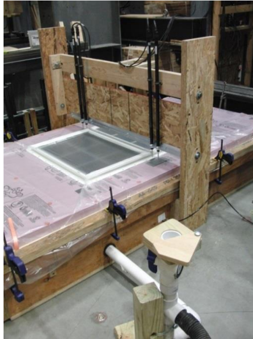
FIGURE 6. WIND PRESSURE LOADING TEST SETUP
