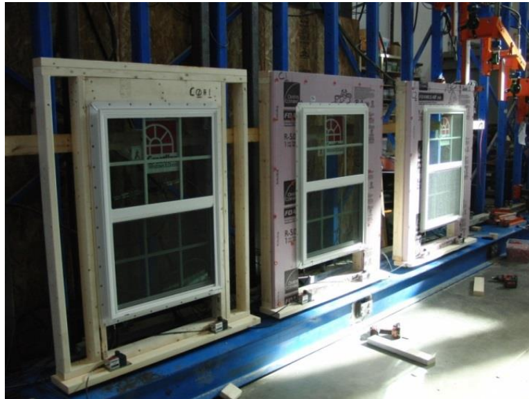
FIGURE 2. LONG-TERM DEFLECTION UNDER SELF-WEIGHT TESTING
